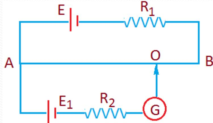
$E = 20 \text{ V}$ ,  $R_{AB} = 20 \Omega$ ,  $R_1 = 5 \Omega$ ,  $R_2 = 5 \Omega$
