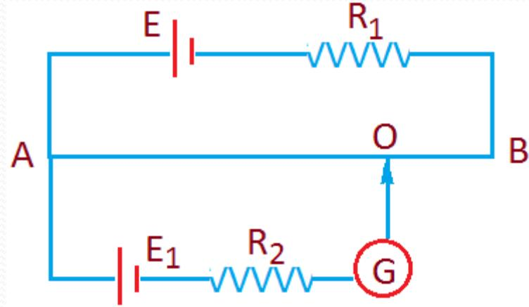
$E = 20 \text{ V}$ ,  $R_{AB} = 10 \Omega$ ,  $R_1 = 6 \Omega$ ,  $R_2 = 5 \Omega$
