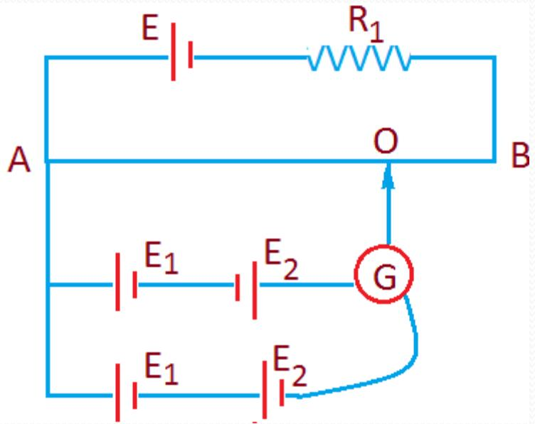
In the figure, a long uniform potentiometer wire AB is having a constant potential gradient along its length. The null points for the two primary cells of emf's  $E_1$  and  $E_2$  connected in the manner shown, are obtained at a distance of 120 cm and 300 cm from the end A. Find (i)  $E_1 / E_2$  and (ii) position of null point for the cell  $E_1$
