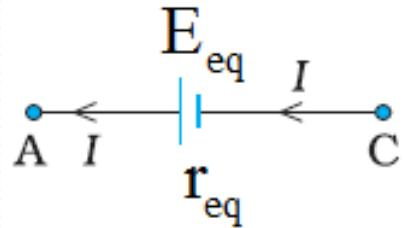
$$V_{AB} = E_1 - Ir_1; \quad V_{BC} = E_2 - Ir_2$$
