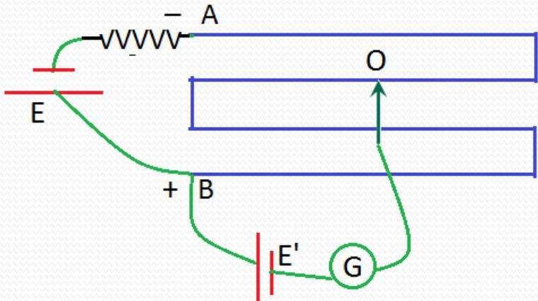
$$E' = V_{BO} \text{ Galvanometer } I' = 0$$
