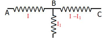
In this circuit also  $V_{AC} = V_{AB} + V_{BC}$  but here  $R \neq R_1 + R_2$  WHY? Is important to note !
