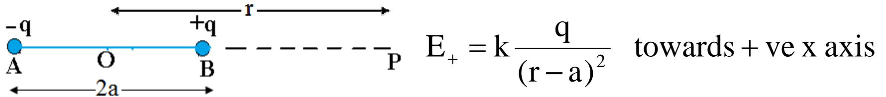
$$E_- = k \frac{q}{(r+a)^2} \text{ towards - ve x axis} \quad \vec{E} = \vec{E}_+ + \vec{E}_- \Rightarrow E_{\text{NET}} = E_+ - E_-$$
