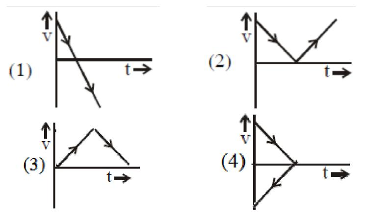
v = u + at; u is positive, a is negative, At highest point v is zero
